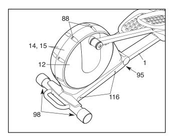
If the elliptical exerciser flexes in the center during use, turn the Center Foot (95) until the flexing is eliminated.
